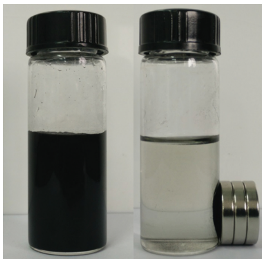
Fig. 5. Separation of MLC-SO 3 H with an external magnet.
