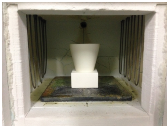
Fig. 3. Photo of lab-scale melting furnace.
