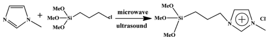
Fig. 1. Scheme for successful synthesis of IL by UMSS method.
