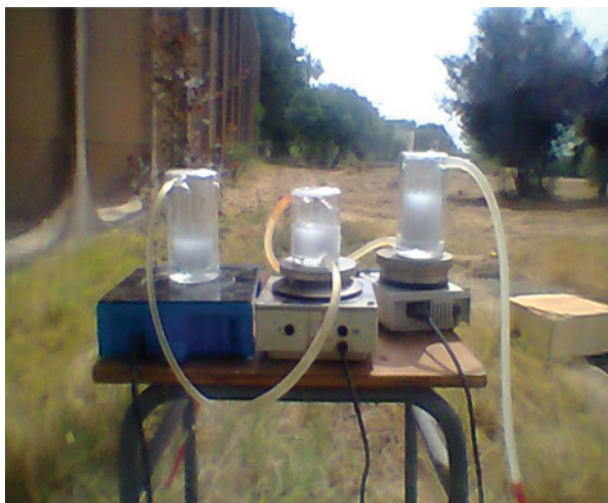
Fig. 1. The experimental set up for the solar photocatalysis.
