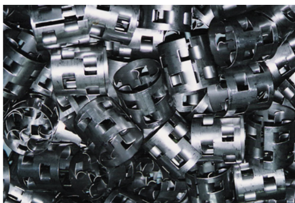
Fig. 5. Column packing: Pall rings.
