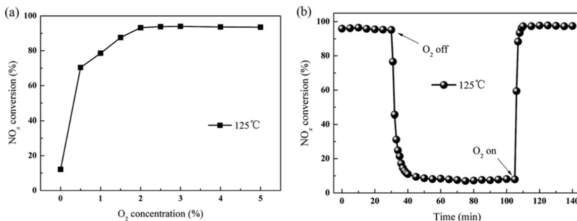
Fig. 7. (a) Effect of  $\text{O}_2$  concentration; (b) Transient response on  $\text{Fe}_{0.7}\text{Mn}_{0.15}\text{Mg}_{0.15}\text{O}_2$  upon switching off and on  $\text{O}_2$ . Reaction conditions:  $[\text{NO}]=[\text{NH}_3]=1,000 \mu\text{L/L}$ , balance  $\text{N}_2$ , total flow rate 2,000 mL/min, catalyst 4 mL, reaction temperature 125 °C.
