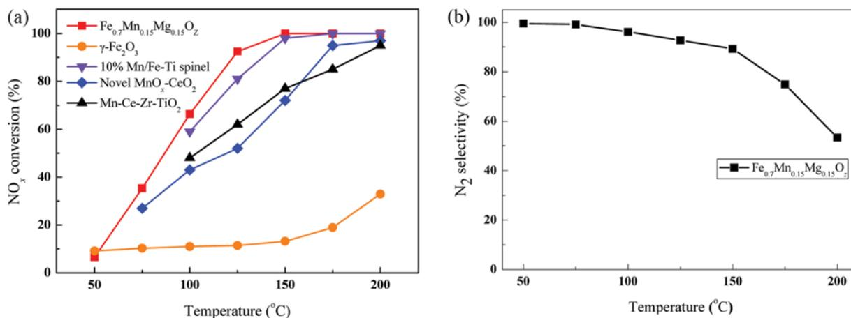
Fig. 1. (a) NO<sub>x</sub> conversion in NH<sub>3</sub> SCR reaction over Fe<sub>0.7</sub>Mn<sub>0.15</sub>Mg<sub>0.15</sub>O<sub>z</sub>, γ-Fe<sub>2</sub>O<sub>3</sub>, 10% Mn/Fe-Ti spinel, MnO<sub>x</sub>(20)/Ce<sub>0.3</sub>Zr<sub>0.7</sub>O<sub>2</sub>(30)-TiO<sub>2</sub> and novel MnO<sub>x</sub>-CeO<sub>2</sub> catalysts; (b) N<sub>2</sub> selectivity of Fe<sub>0.7</sub>Mn<sub>0.15</sub>Mg<sub>0.15</sub>O<sub>z</sub> catalyst.
