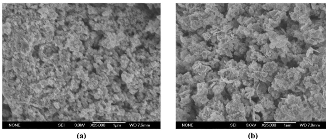
Fig. 4. (a) SEM photo of  $\gamma\text{-Fe}_2\text{O}_3$ ; (b) SEM photo of  $\text{Fe}_{0.7}\text{Mn}_{0.15}\text{Mg}_{0.15}\text{O}_z$ .
