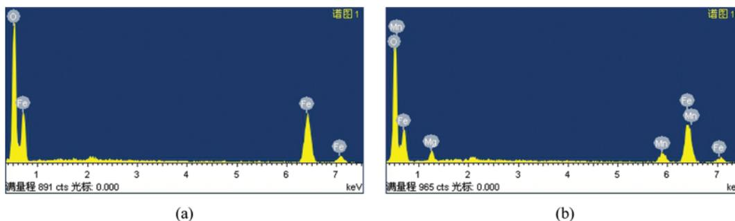
Fig. 5. (a) EDS spectra of  $\gamma\text{-Fe}_2\text{O}_3$ ; (b) EDS spectra of  $\text{Fe}_{0.7}\text{Mn}_{0.15}\text{Mg}_{0.15}\text{O}_z$ .
