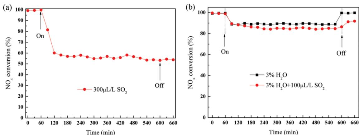
Fig. 8. (a) Effect of SO<sub>2</sub>; (b) Effect of SO<sub>2</sub> and H<sub>2</sub>O. Reaction conditions: [NO]=[NH<sub>3</sub>]=1,000 μL/L, [O<sub>2</sub>]=3.5%, balance N<sub>2</sub>, total flow rate 2,000 mL/min, catalyst 4 mL, reaction temperature 150 °C.
