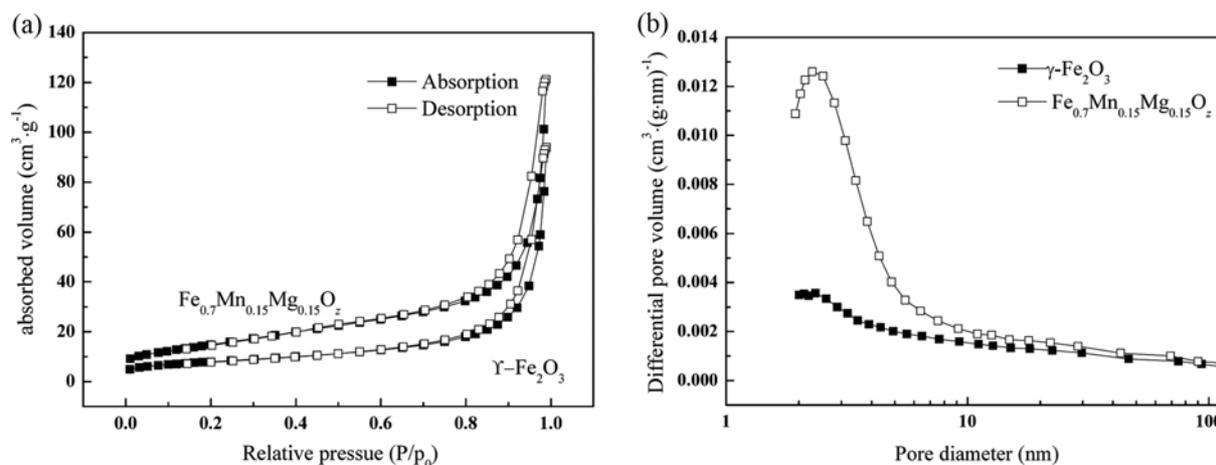
Fig. 3. (a) N<sub>2</sub> adsorption-desorption isotherms; (b) BJH desorption pore size distribution plots of  $\gamma$ -Fe<sub>2</sub>O<sub>3</sub> and Fe<sub>0.7</sub>Mn<sub>0.15</sub>Mg<sub>0.15</sub>O<sub>2</sub> catalysts.
