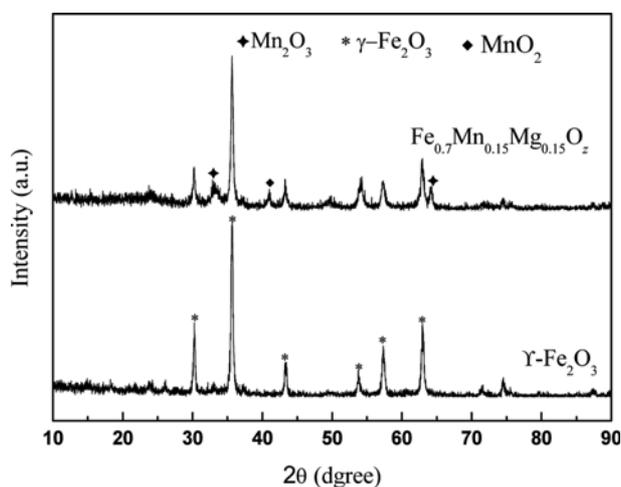
Fig. 2. XRD patterns of Fe<sub>0.7</sub>Mn<sub>0.15</sub>Mg<sub>0.15</sub>O<sub>z</sub> and γ-Fe<sub>2</sub>O<sub>3</sub> catalysts.
