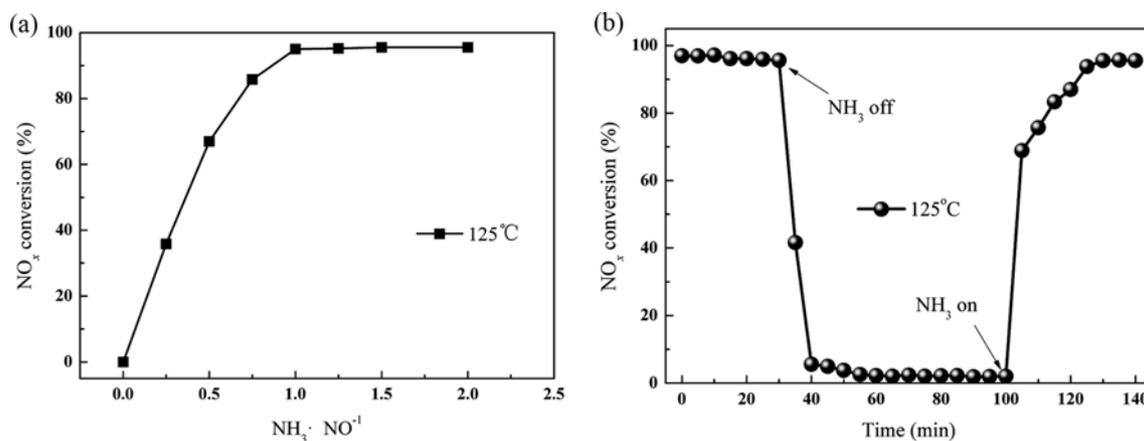
Fig. 6. (a) Effect of  $\text{NH}_3/\text{NO}$  concentration; (b) Transient response on  $\text{Fe}_{0.7}\text{Mn}_{0.15}\text{Mg}_{0.15}\text{O}_2$  upon switching off and on  $\text{NH}_3$ . Reaction conditions:  $[\text{NO}]=1,000 \mu\text{L/L}$ ,  $[\text{O}_2]=3.5\%$ , balance  $\text{N}_2$ , total flow rate 2,000 mL/min, catalyst 4 mL, reaction temperature 125 °C.
