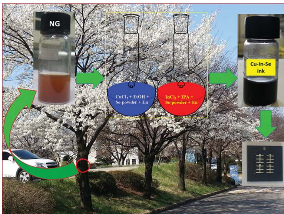
Fig. 1. Schematic of CIGSe solar cell fabrication using cherry blossom tree gum assisted binary Cu-Se and In-Se NPs ink.
