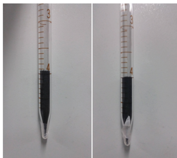
Fig. 2. Volumetric measurement (left: original coal; right: pretreated coal, 0.6 g respectively).
