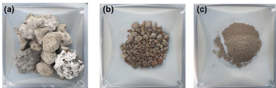
Fig. 1. Photo images of initial SS (a) before and (b) after crushing by hammer mill and (c) after crushing by ball mill.
