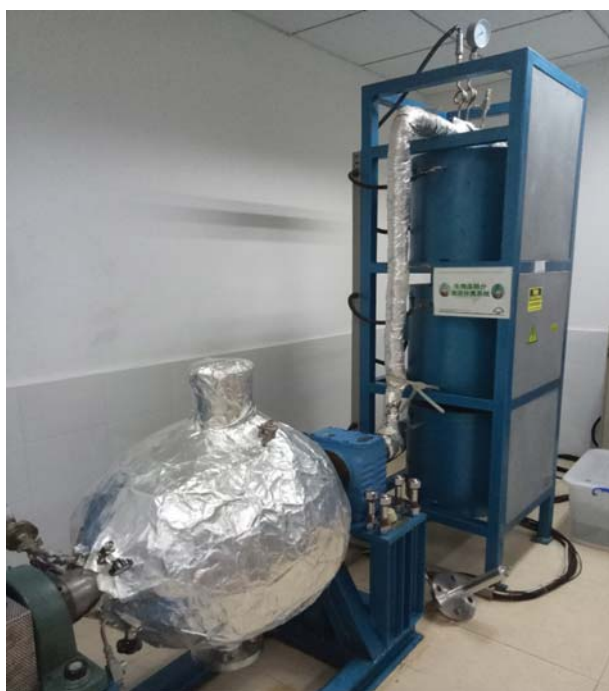
Fig. 1. Ball-shaped reactor for the production of cellulosic pulp by CAOSA process.
