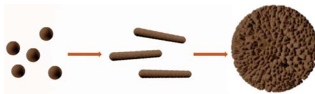
Fig. 1. Schematic of formation mechanism of \text{Gd}^{3+} -doped \text{WS}_2 particles.
