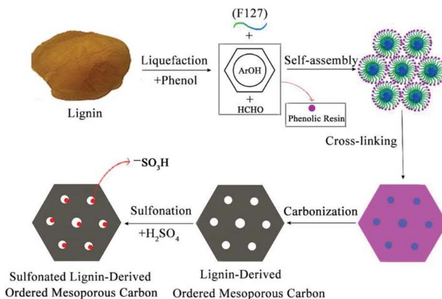
Scheme 2. Schematic illustration of the synthesis process of sulfonated lignin-derived ordered mesoporous carbon derived from kraft lignin.
