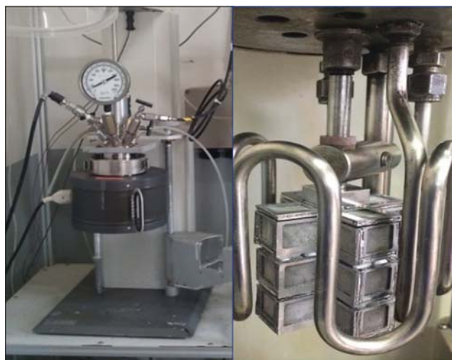
Fig. 1. Parr autoclave 1-L batch reactor and baskets for catalysts inside a batch reactor.
