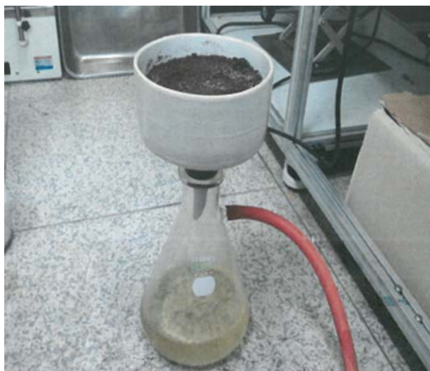
Fig. 2. Apparatus for the clay filtration as an aspirator.
