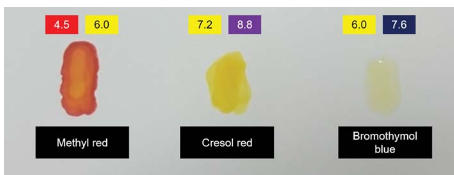
Fig. S2. Photographs of pH test of Epson photo paper. Methyl red (red at pH 4.4 to yellow at pH 6.0), cresol red (yellow at pH 7.2 to purple at pH 8.8) and bromothymol blue (yellow at pH 6.0 and blue at pH 7.6) have used for pH testing. Based on the indicator test, the pH of the photo paper is estimated to be less than 4.4.
