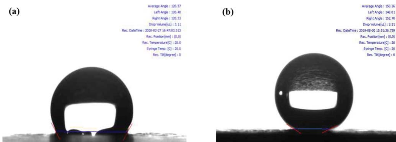
Fig. 3. Contact angle of water with (a) CP (SGL 29AA) and (b) MPL/CP (SGL 29BC).
