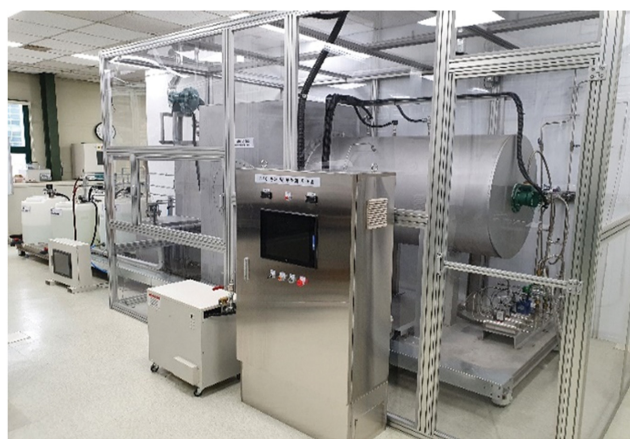
Fig. 2. Combustion based SF 6 decomposition and pollution control system. (a) Schematic diagram of the pilot system, (b) Photograph of the pilot system.
