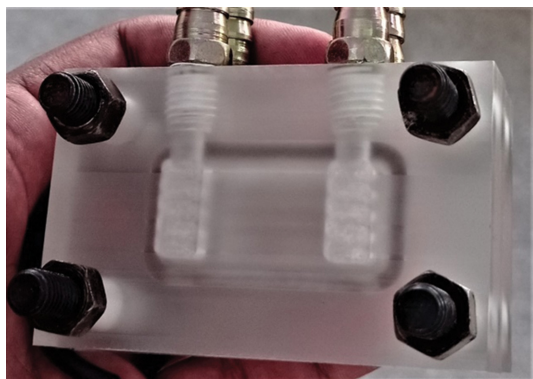
Fig. 2. Locally fabricated FO module for inorganic membrane testing.
