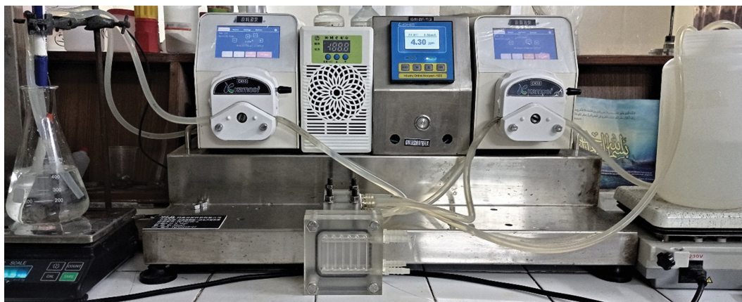
Fig. 1. FO bench-scale apparatus.
