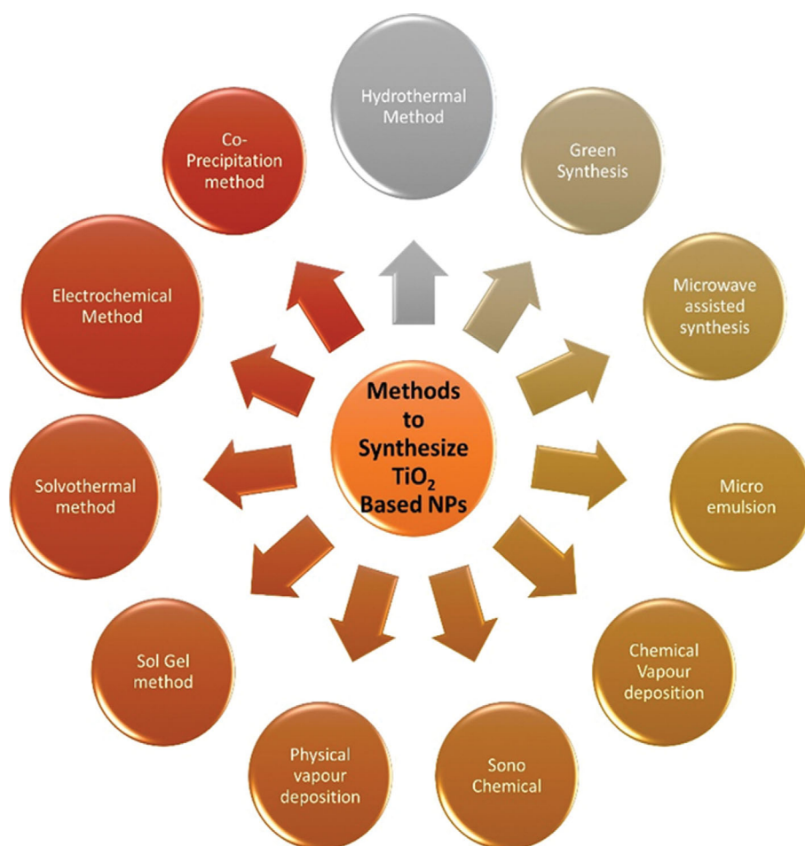
Fig. 1. Methods used to synthesize TiO 2 and TiO 2 based materials.
